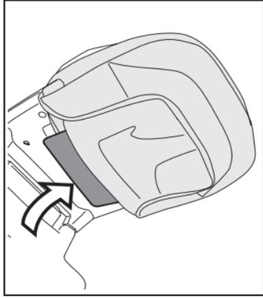
**2.** Slip the seat lining on from the front (fig\_a), inserting the profile in the appropriate slot (fig\_b).
