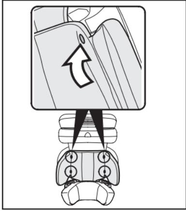
**8.** Slightly raise the headrest and put the lining back in place, fastening the two elastics as shown, first on one side (fig\_a) and then on the other (fig\_b), and paying attention to the white polystyrene.
