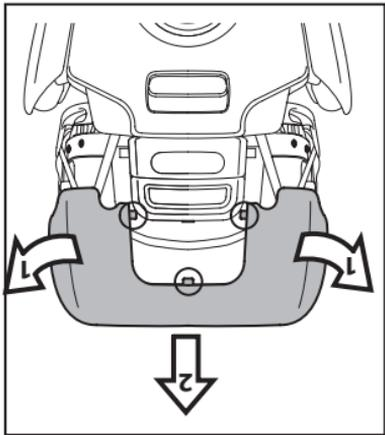
**10.** To remove the headrest upholstery, slightly raise the headrest, and release the two elastic bands on one side (fig\_a) and then on the other (fig\_b). Remove the upholstery.
