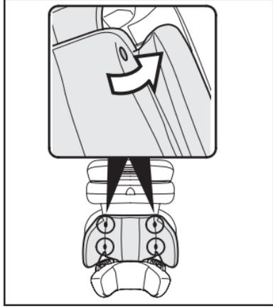
6. Release the two upper elastic bands and the two lower ones located on each side.
