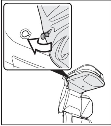
**4.** Finally, attach the two side eyelets to the buttons on the sides of the seat.
