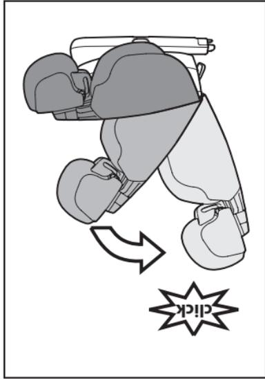
**1.** Raise the car seat backrest until it clicks; the product should remain upright on its own. The backrest oscillates by a few degrees to better fit the different types of vehicle seats.
