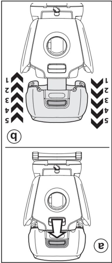
Viaggio Flex 120 adjusts to grow with your child. Each adjustment is independent to ensure maximum flexibility of use. 1. The headrest can be adjusted in 5 positions. Lift the handle (fig\_a) on the back of the headrest and simultaneously raise the headrest (fig\_b), placing it at the desired height.
